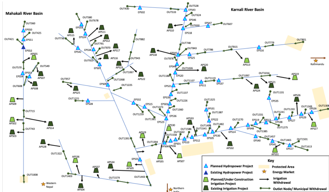
Figure 17: Schematic of the node system used in the Western Nepal application.
