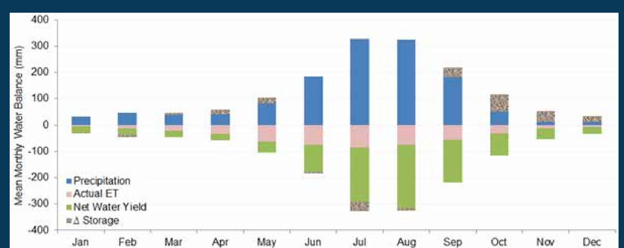
Figure 4: Mean monthly simulated (1995-2009) water balance in the KarMo basin. storage is a collective term including groundwater recharge and change in soil moisture storage.
