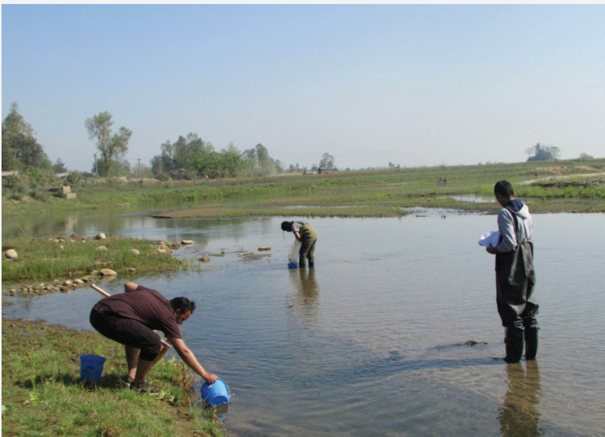
Sampling of benthic macroinvertebrates in a 50- to 100-meter stretch of river.
